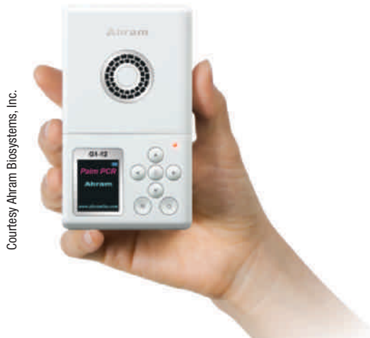
Figure 9.9 This handheld PCR machine will allow samples to be processed and analyzed at the crime scene.
